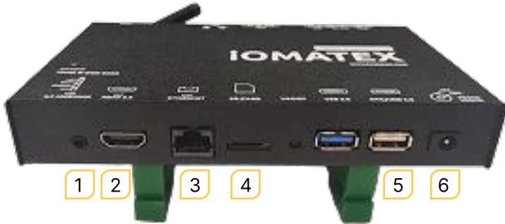
Figure 3. Front view of the interfaces of the IOMX G-Box 023D network gateway
