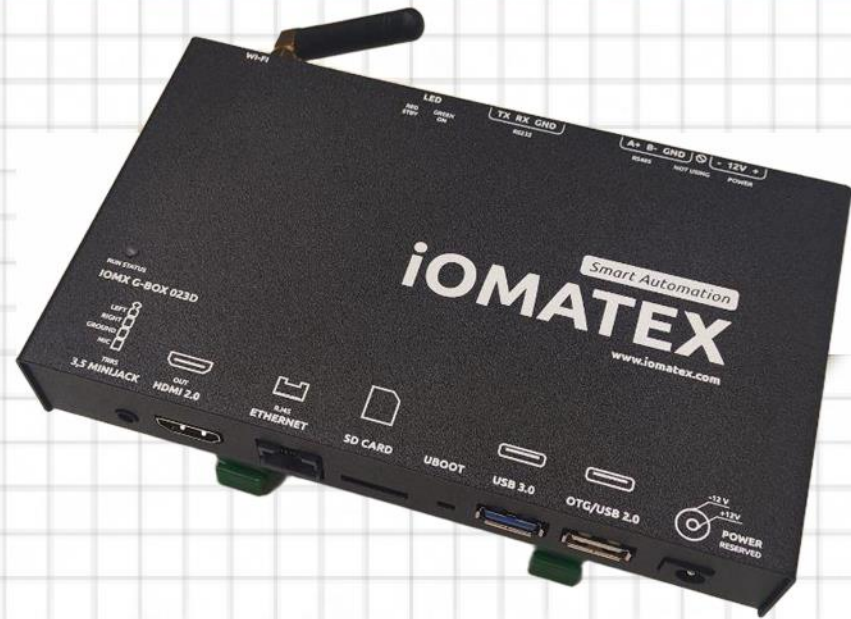
1. Main Central Microprocessor Unit & Wi-Fi Antenna
